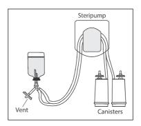
Pic. 5: Schematic Set-up of Stericheck SVP1
